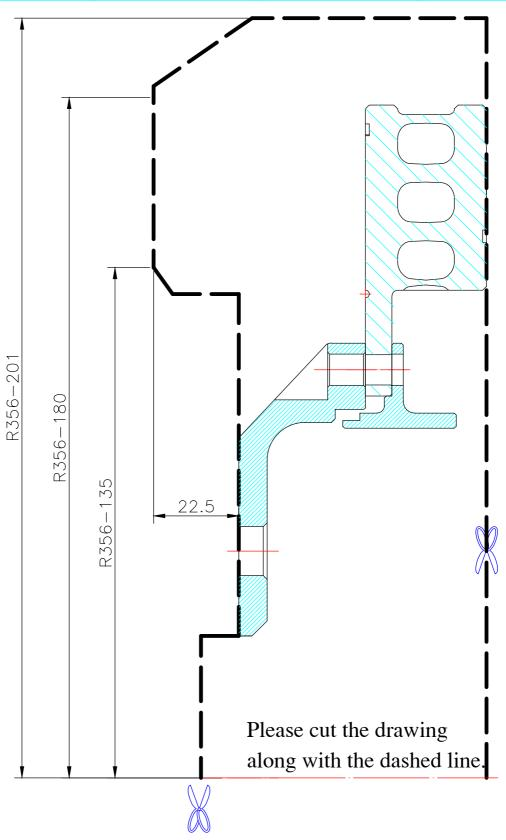
The wheel fitment is only for your reference and it can not 100% ensure the clearance between caliper and rim is ok. if there is any interference issue, please change your wheel as possible.
